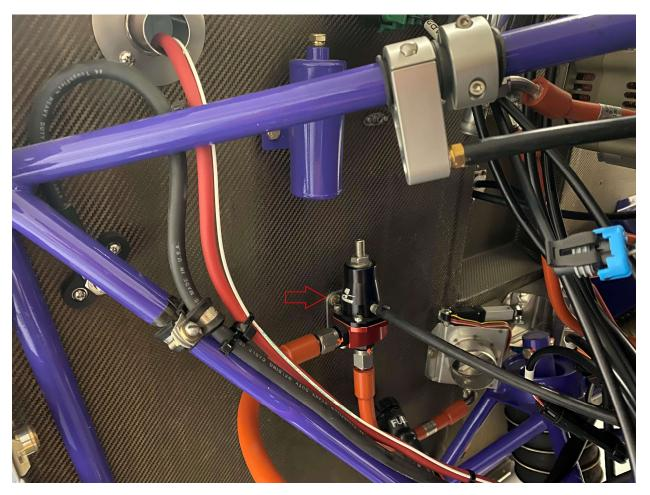
the regulator on the firewall at the approximate location shown here. After loosely attaching these hoses, you can mark the final location to the mount the regulator on the firewall.
